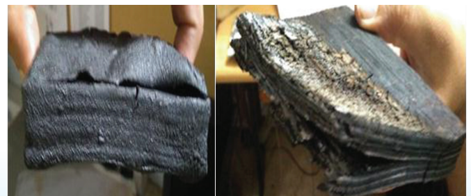
Coated v/s bare wood specimen at 400°C
